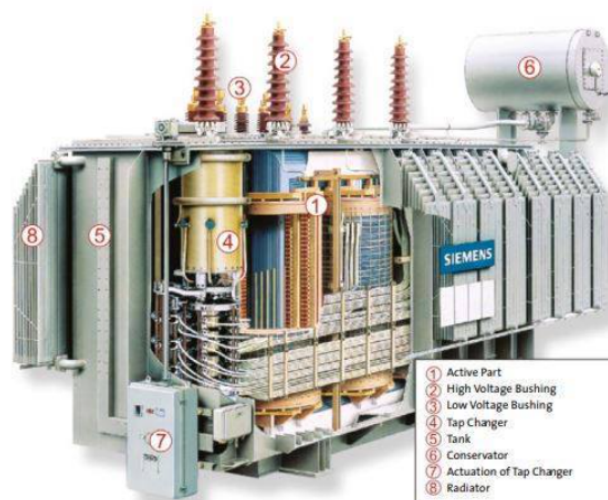
Figure 2.1: PT labeled with some of the most important components [29]
